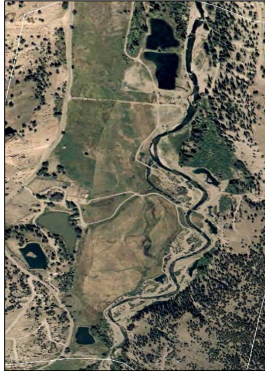
Photo 9-2: Lake Fork River in October 2005 (image by USDA Farm Service Agency via Google Earth). A large channel stabilization project was completed some time between 1998 to 2005. The project increased the channel sinuosity, narrowed the channel width, and installed many cross vanes and J-hooks throughout the reach. The project objectives were to improve fisheries. A bridge was installed across the river and a picnic pavilion was later built immediately downriver from the bridge.
