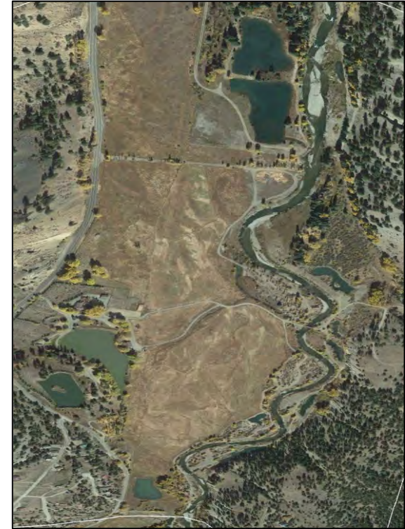
Photo 9-3: Lake Fork River in October 2015 (image by Google Earth). Notice that the channel width has increased throughout the reach. Which combined with decreased water depth likely reduces habitat quality. Sediment deposition has buried at least two cross vanes on the lower portion of the reach. It also appears that this sediment deposition has affected the performance of the diversion structure used to fill the ponds near the bottom of the reach. Access roads developed during construction remain and likely limit floodplain connectivity within the reach.
