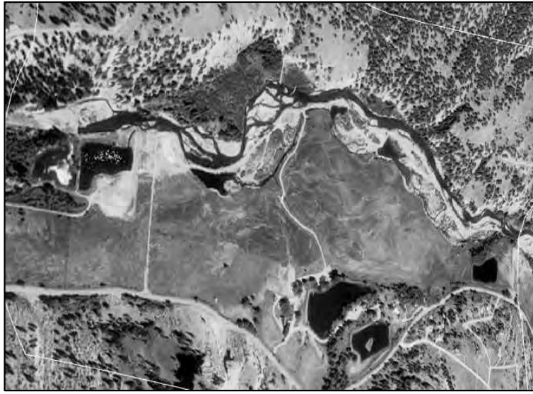
Photo 9-1: Lake Fork River in September 1998 (image by USGS via Google Earth). In the center of the image multi-thread channels navigate large, wide sediment deposits. A low-water ford allowed vehicles to cross the river. Prior stream stability and channels configurations are unknown.
