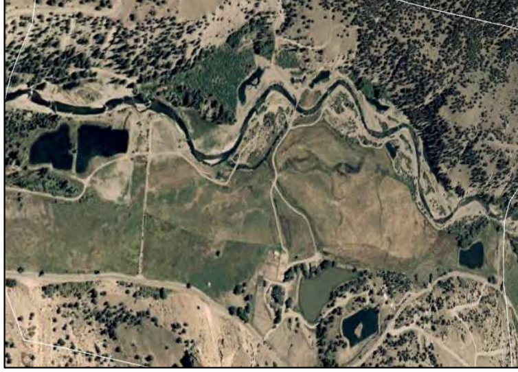
Photo 9-2: Lake Fork River in October 2005 (image by USDA Farm Service Agency via Google Earth). A large channel stabilization project was completed some time between 1998 to 2005. The project increased the channel sinuosity, narrowed the channel width, and installed many cross vanes and J-hooks throughout the reach. The project objectives were to improve fisheries. A bridge was installed across the river and a picnic pavilion was later built immediately downriver from the bridge.
