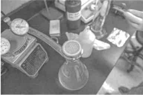
Algae collects on a filter. The door and shades in the room were closed while the team prepared samples to prevent the algae from continuing to grow.
