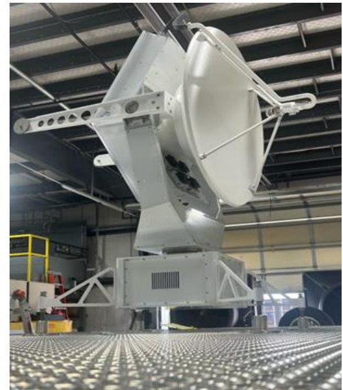
The Doppler radar unit which will be temporarily mounted on a thirty-foot trailer.
